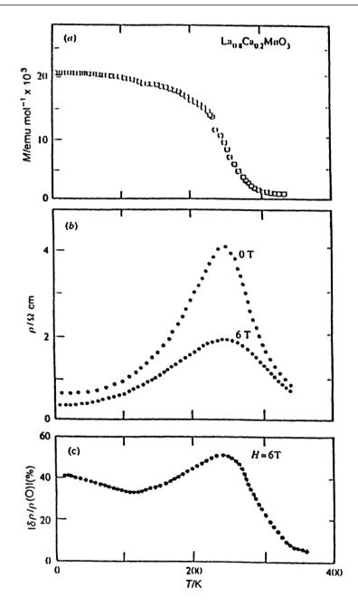
Fig. 2: Temperature-variation of (a) the magnetization, (b) the resistivity (at 0 and 6T) and (c) the magneto resistance in  $La_{0.8}Ca_{0.2}MnO_3$ .
