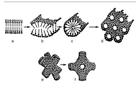
Fig. 4: Phase transitions in mesoporous solids: a-d : lamellar-hexagonal, e-f, hexagonalcubic. The circular objects around the surfactant assemblies one metal-oxo species.
