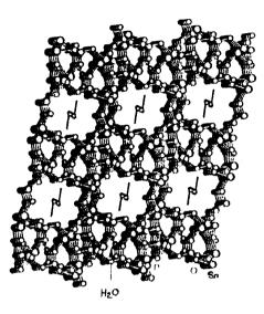
Fig. 3: Structure of a open-framework metal phosphate synthesized hydrothermally in the presence of an organic amine template.
