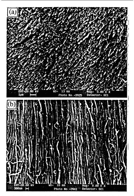
Fig. 6: Aligned carbon nanotube bundles. (a) and (b) are in two perpendicular directions.
