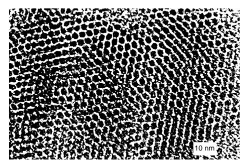
Fig. 5: Thiolised Pd<sub>561</sub> nanoparticle array.
