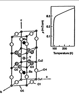
Fig. 1: Superconducting YBa<sub>2</sub>Cu<sub>3</sub>O<sub>7</sub>.
