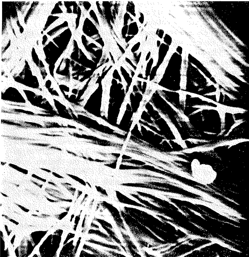
FIG. 8 — Electron micrograph of a sample of fibrous cerium (IV) phosphate (Magnification 10,000 X).
