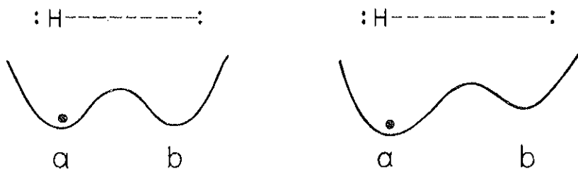
FIG. 17 — Typical double-well potentials felt by a proton in a hydrogen bond; the left-hand potential is symmetric, and the right-hand potential is asymmetric.
