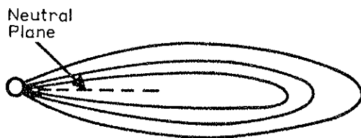
FIG. 1 — Magnetic bulge with neutral plane.
