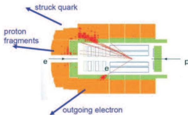
Figure 2: Schematic view of the H1 experiment and, superimposed, a neutral current event. The scattered electron, the particle shower resulting from the struck quark and traces of the proton fragments are clearly visible
