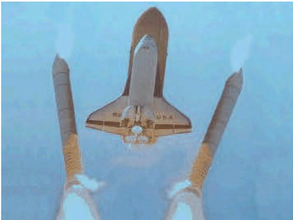
Figure 32: Separation of the Solid Rocket Boosters.
