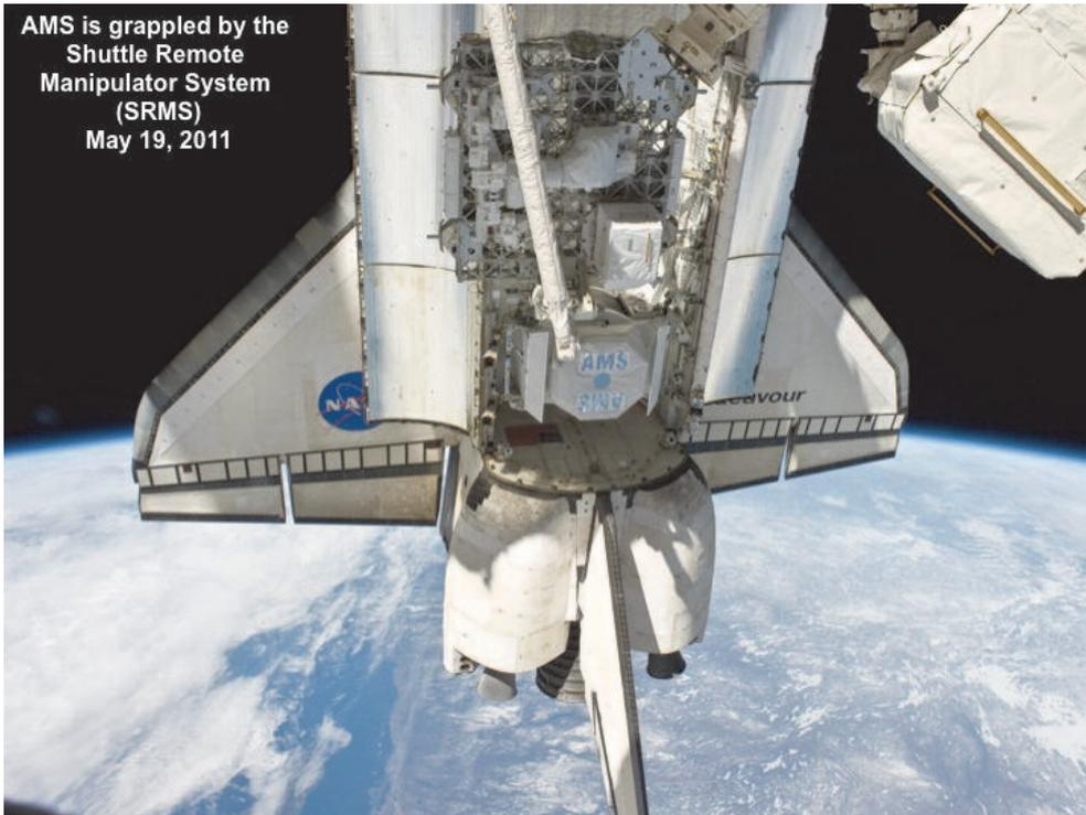
Figure 37: After docking with the ISS, AMS was removed from *Endeavour's* cargo bay by the shuttle Remote Manipulator System and transferred to the ISS robotic arm that placed AMS on its permanent attachment site on an external truss of the ISS.
