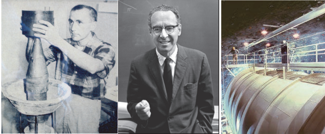
Figure 7. a) (left) Lee Grodzins c. 1957 holding the magnet of the experimental apparatus for analyzing the circular polarization of \gamma -rays detected by resonant scattering. The difference in counting rate due to reversing the magnetic field measures the circular polarization. The \text{Eu}_2\text{O}_3 source is inside the center of the magnet. The cone is a Pb absorber which restricts the path of the circularly polarized \gamma -rays from \text{Sm}^{152*} decay so that they pass through the magnetized iron on their trajectory to the basin at the bottom which is the \text{Sm}_2\text{O}_3 resonant-scatterer. The re-emitted \gamma -rays are detected in a scintillation counter under the Pb cone. b) (center) Maurice Goldhaber c. 1967. c) (right) Ray Davis' tank of cleaning fluid in the Homestake mine 1967. All photos courtesy BNL.
