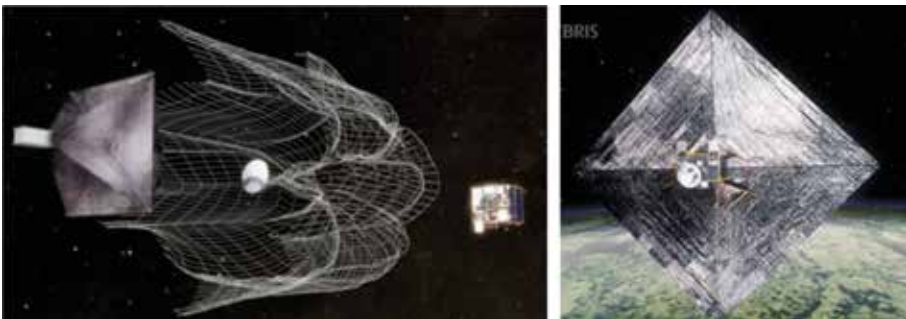
Figure 6. In-orbit assembly of a large aperture from individual microsatellites.
