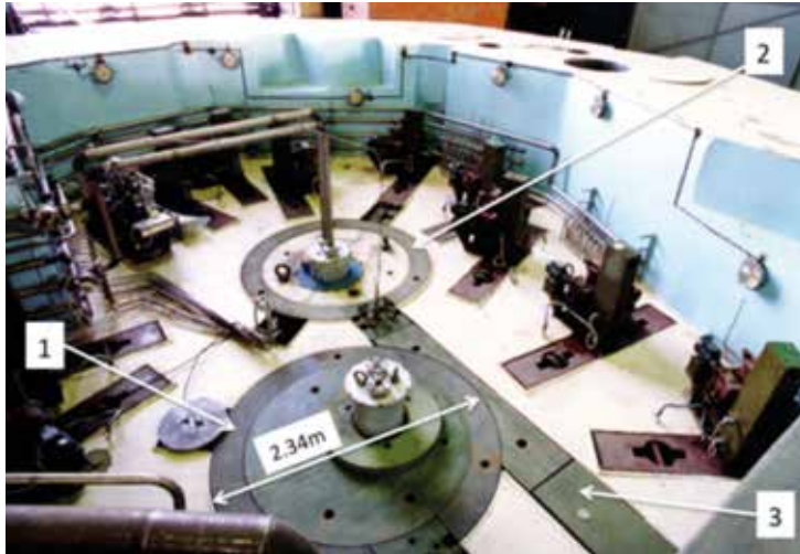
Figure 11. Photograph of the INR Troitsk beam target area showing the proposed ADS pit (1), the presently operating pulsed neutron source cell (2), and its beam line (3). Taken from [38].
