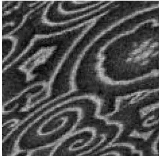
Figure 16. PEEM image ( 0.36 \times 0.36 \text{ mm}^2 ) from a Pt(110) surface in the state of chemical turbulence during catalytic CO oxidation at T=548 \text{ K} , p_{\text{CO}}=1.2 \times 10^{-4} \text{ mbar} .
