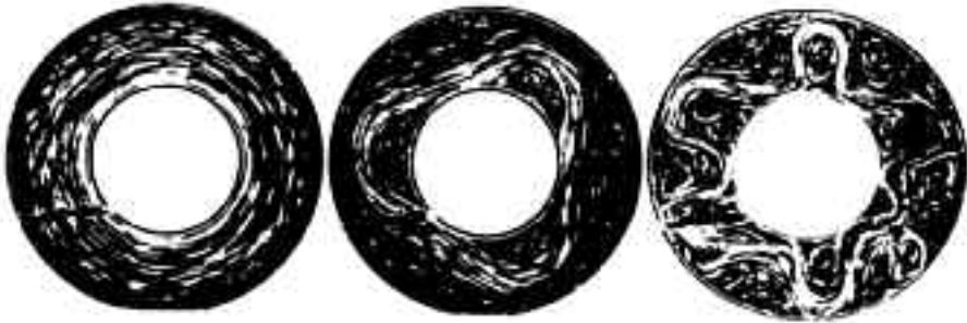
Figure 1. Streak photographs taken to illustrate three typical top-surface flow patterns, the first in the axisymmetric régime, the second in the regular non-axisymmetric régime (of 'vacillation') with M=3 , and the third in the irregular ('chaotic') non-axisymmetric régime (of 'geostrophic turbulence'). The respective values of \Omega were 0.34, 1.19 and 5.02 radians per second; other impressed conditions were held fixed.
